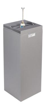
EMR Band Pass Cavities are 1/4 wavelength, high Q cavity filters with excellent selectivity. Bandpass cavities reject frequencies outside of a narrow pass band. These cavities may be factory tuned to specific frequency and are field tunable. Multiple cavities may be connected for greater selectivity with minimal insertion loss and wider pass bandwidths. Multi-cavity configurations come standard with 19 inch EIA rack mounting bars or panel with chassis tray.
