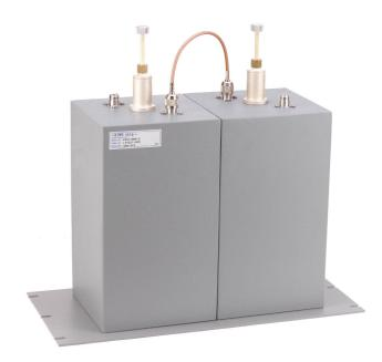
EMR Band Pass Cavities are 1/4 wavelength, high Q cavity filters with excellent selectivity. Bandpass cavities reject frequencies outside of a narrow pass band. These cavities may be factory tuned to specific frequency and are field tunable. Multiple cavities may be connected for greater selectivity with minimal insertion loss and wider pass bandwidths. Multi-cavity configurations come standard with 19 inch EIA rack mounting bars or panel with chassis tray.
