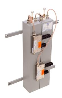
EMR Filter-Ferrite Transmitter Combiners use space saving, High-Q square cavity resonators, and wideband isolators providing lower insertion loss than hybrid designs. Standard units are mounted to a 19 inch EIA rack. Multiple mounting and free standing configurations available.
