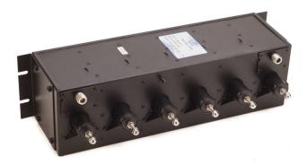
The 5044-8 Band Pass Filters are 6-cavity devices which provide band pass characteristics for both transmitter and receiver applications in the 800 MHz frequency bands. This product utilizes the superior RF conductivity of copper for excellent performance. The 5044-8 Series is capable of power requirements that average 600 watts. Both types of filters employ adjustable aperture coupling between resonators that are permanently fixed at the factory.
