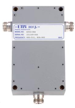
EMR 6050 Series Crossband Coupler uses aluminum alloy outdoor enclosure with 3 type N Female RF connectors and a standardized 3 inch x 5 inch mounting footprint. The coupler versions of this product line allow two separate 125 Watt VHF or UHF transmitters to be used with one multi-band or broadband antenna, saving transmission line cost and cable plenum space.
