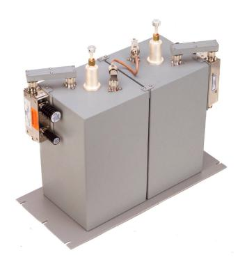
EMR Filter-Ferrite Transmitter Combiners use space saving, High-Q square cavity resonators, and wideband isolators providing lower insertion loss than hybrid designs. Standard units are mounted to a 19 inch EIA rack. Multiple mounting and free standing configurations available.
