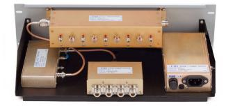
EMR Receiver Multicouplers allow several receivers to share a common antenna. These units include a preselector, amplifier, power supply and power divider which effectively amplifiy a filtered band of frequencies to individual receivers. The power divider provides a minimum of 23 dB of port-to-port isolation preventing signal mixing even at minimal channel separation.
