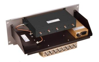
EMR Receiver Multicouplers allow several receivers to share a common antenna. These units include a preselector, amplifier, power supply and power divider which effectively amplifiy a filtered band of frequencies to individual receivers. The power divider provides a minimum of 23 dB of port-to-port isolation preventing signal mixing even at minimal channel separation.
