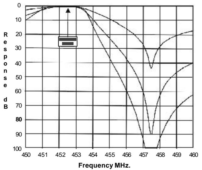
Responses of one, two and three series pass reject UHF 4" square cavities @ 5 MHz. spacing.
