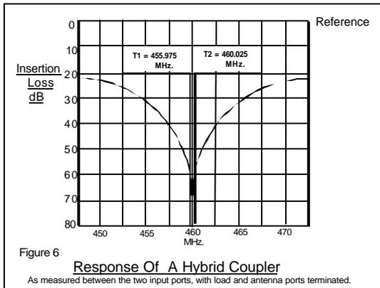
This effect is demonstrated in Figure 6. There are two very closely spaced transmitter frequencies, 459.975 and 460.025 MHz to be combined. Note that we phase the hybrid on the mean frequency 460.000 MHz. The dark vertical lines represent the two transmit frequencies.
