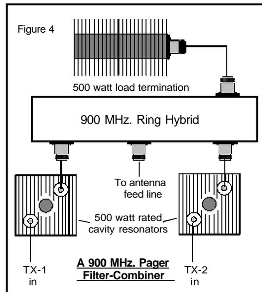
Figure 4 shows an example using the ring hybrid coupler. This is a combiner for two 930 MHz Band 500 watt paging transmitters together with additional filtering provided by the series band pass cavity resonators. It is a good
