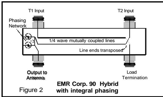
The strip lines are transposed at one end to facilitate the best chassis layout for a Hybrid – Ferrite transmitter combiner. Note that the T1 and T2 input connectors are on the same side of the hybrid housing. We have also included a network at the antenna port that when properly adjusted, will produce more than 65 dB of isolation between the T1 and T2 input ports.
