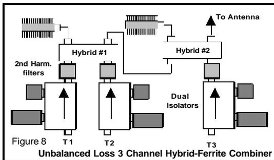
Where uniform *per channel* losses are not important, a two hybrid arrangement can be used as shown schematically in Figure 8.
