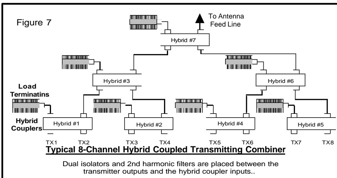
cable, connector and residual losses in the hybrid itself. In system design work we use 3.2 dB per split which turns out to be quite close in practice.
