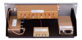
EMR Receiver Multicouplers allow several receivers to share a common antenna. These units include a preselector, amplifier, power supply and power divider which effectively amplifiy a filtered band of frequencies to individual receivers. The power divider provides a minimum of 23 dB of port-to-port isolation preventing signal mixing even at minimal channel separation.
