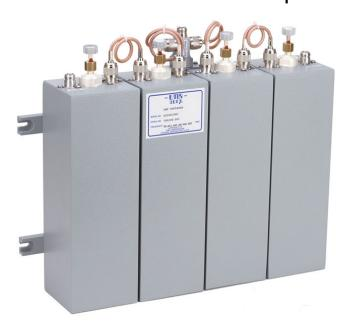
EMR band-pass duplexers allow for the simultaneous use of a transmitter and receiver on a single common antenna. Band pass cavities allow a specific frequency or group of frequencies (pass band) to pass through the device while providing rejection against all other frequencies. Our signature square cavities provide greater Q while requiring less space than conventional round cavities.
